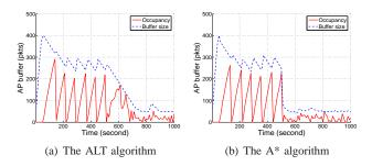
Fig. 13. Convergence rate of the ALT and  $A^*$  algorithms. One download flow,  $a=10,\,b=1.$  At time 500s the number of upload flows is increased from 0 to 10.
